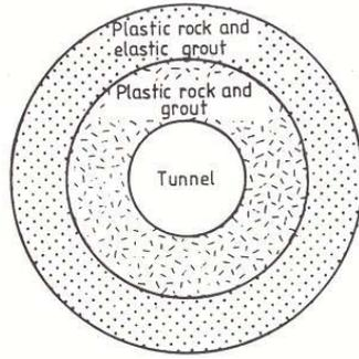
**Figure 8. Rock and grout conditions in the rock mass**
