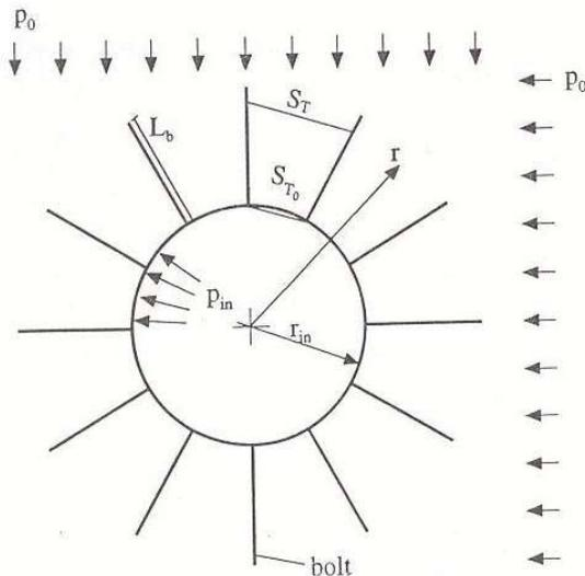
**Figure 17. Geometry of the axisymmetric problem (after Oreste & Peila,1996).**
