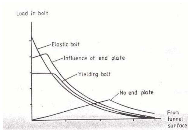
**Figure 10. The different analytic bolt load distributions of a grouted bolt.**
