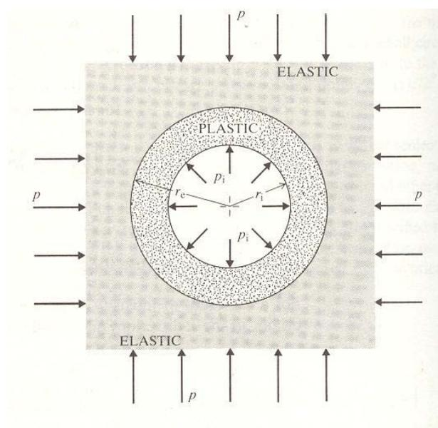
**Figure 16. Assumed opening geometry (after Brady & Beown, 1985).**
