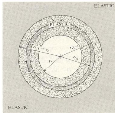
**Figure 18. Plastic zone divided into thinannuli for finite difference solution (stepwise geometrical discretization) (after Brady & Brown,1985).**
