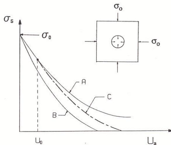
**Figure 15. Effect of grouted bolts on ground convergence curve ((after Intraratna, 1987,1990)**
