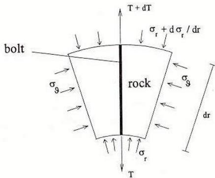
**Figure 20. Stresses in the bolt and in the rock mass(after Oreste &Peila,199).**
