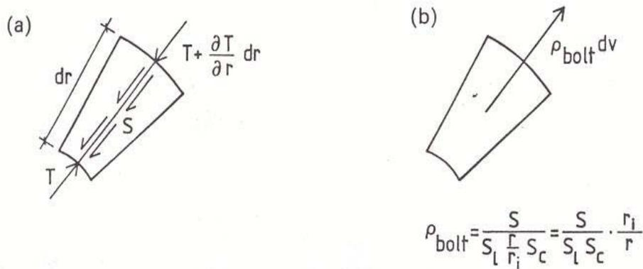
**Figure 7. Stresses in the bolt and rock at plastic deformation in the grouting material (a) Stresses in the bolt. (b) Stresss in the rock.**
