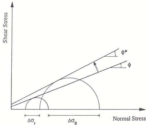
**Figure 14. Effect of grouted bolts on failure envelope (after Intraratna, 1987,1990)**
