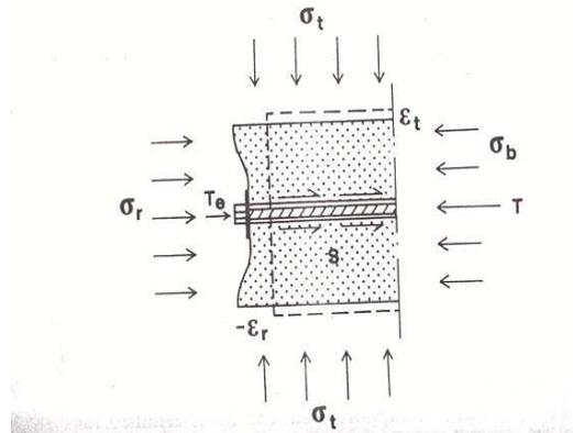
**Figure 9. Interaction between rock mass and bolt with end plate. Local deformations of the rock mass under the end plate is shown.**
