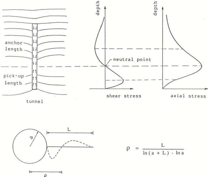
Figure 11. Stress distribution model for grouted bolts (after Xueyi, 1983).
