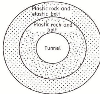
**Figure 6. Rock and bolt conditions in the rock mass**
